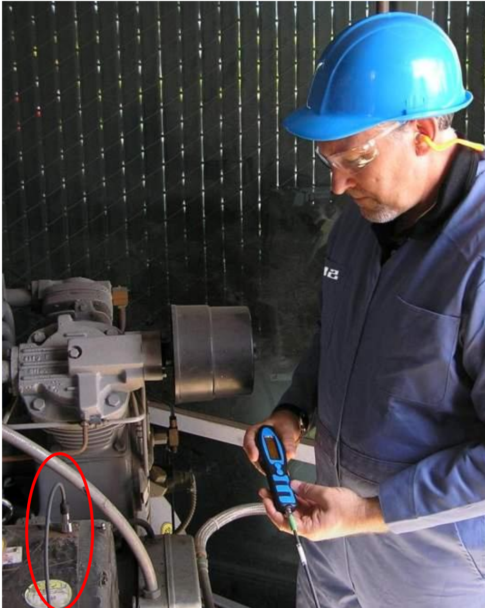
Standard ICP accelerometers with 100 mV/g, CMAC107
